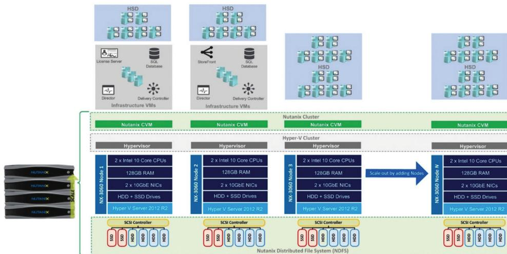
Figure 3. Logical View of the RDSH Solution
