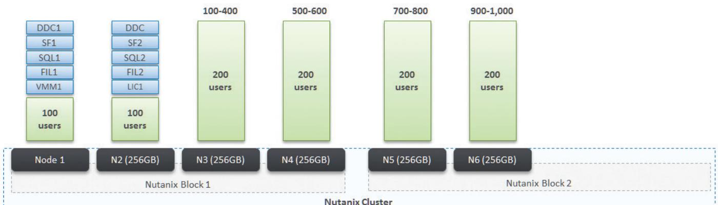
Figure 7. 1,000 RDSH Users - Virtual Machine allocation in relation to Nutanix Node
