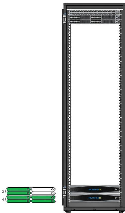
**Figure 13. Rack Layout – 6 x Nodes**
