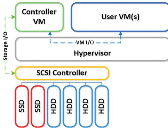
Figure 6. Logical View of a Nutanix Node
