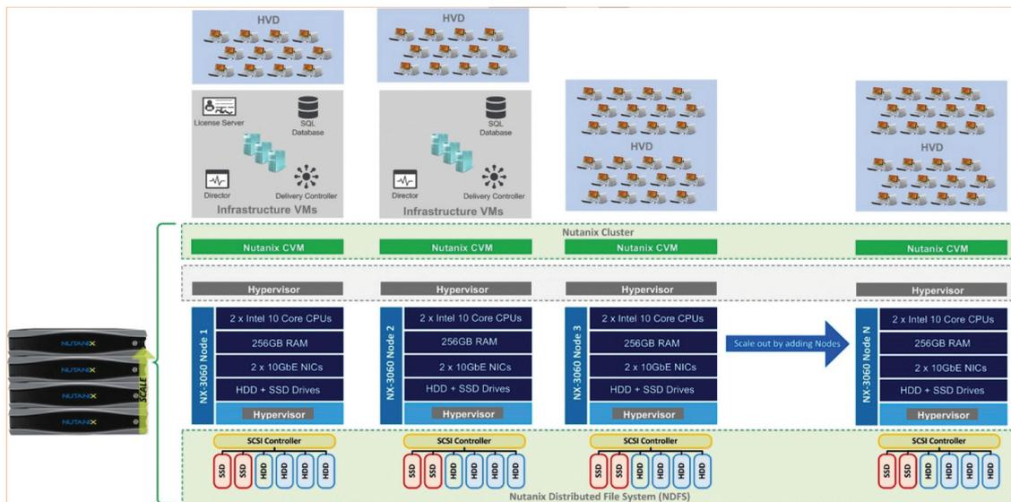
Figure 4. Logical View of the HVD Solution
